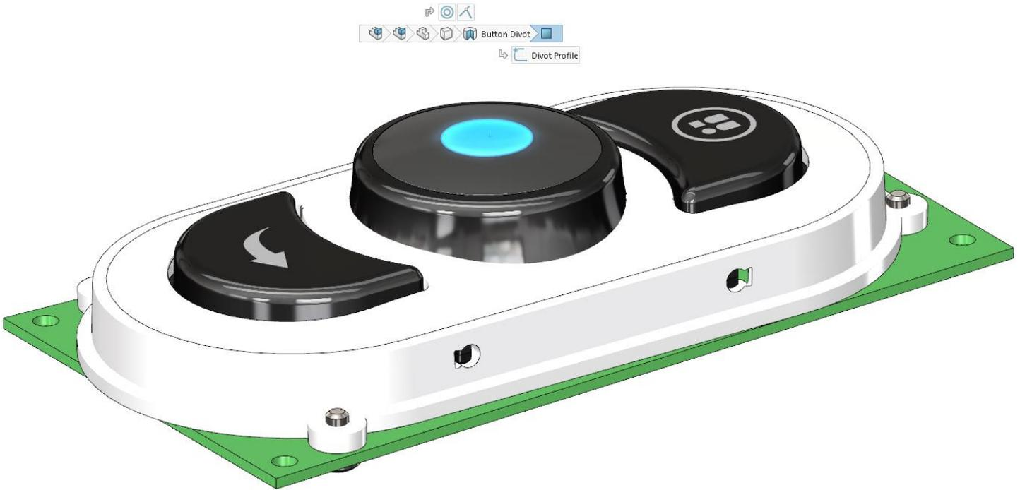
We have access to additional information including mates and the ability to select any sub assembly levels along with the top level assembly, should we wish to open or modify those. Hovering over the mates show a preview of the selected surfaces and can be directly edited from a right click on the area you wish to edit/ open.
